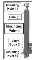
**Mounting Hole #2, right)**, securing it as well. Make sure the pins' diameters are a push fit with just enough clearance so they move freely. The pins should be held in place with appropriate e-clips or hardened cotter pins (neither one included).
